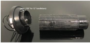
STEP 4: Cut the locking tabs off of the throttle assembly .500-.600" from the housing.
