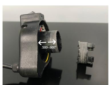
STEP 5: Cut the tabs off one outside end of only one of the ODI grips and sand smooth.
