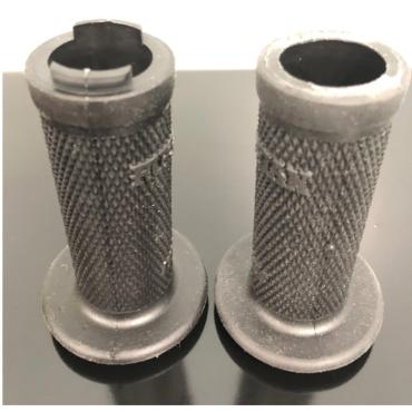
STEP 6: Install the adapter on the ODI grip that you cut the tabs off of the outside end and check to make sure it rotates smooth on the handlebars. If it has any resistance lightly sand the inside of the locking tabs and test again.
